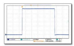
Pulsed current: 100Apk, 21µs Ch1-CWT (300A) Ch2-Co-ax shunt 2GHz Timebase 4µs/div
