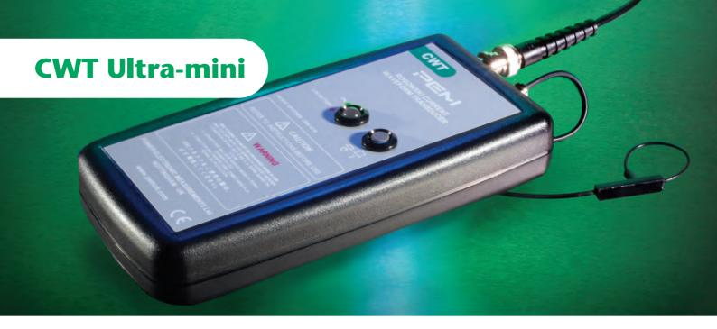
The CWT Ultra-mini has an extremely thin, clip-around Rogowski coil of typically 1.6mm cross-section. Such a thin coil enables currents to be measured in the most difficult to reach parts of a power electronic converter with negligible disruption to the circuit under test.
